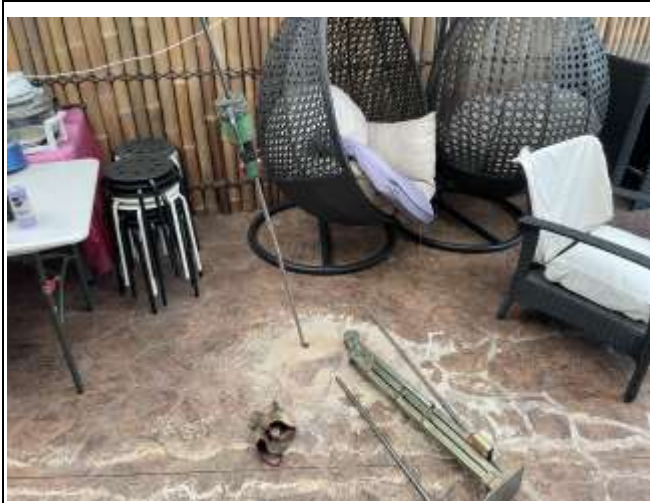
Photograph 1 Dynamic Cone Penetrometer(DCP) at location of DCP2 at rear portion
